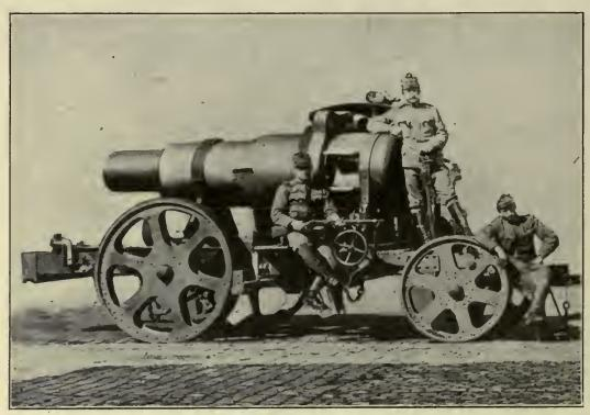
ONE OF THE FAMOUS GERMAN SIEGE GUNS. [Newspaper Illustrations.] This photograph shows part of gun mounted on a special trolley to facilitate transport. The photograph below illustrates the lower mounting of the gun, with recoil cylinders. The gun is mounted up and placed on a concrete foundation for firing.
